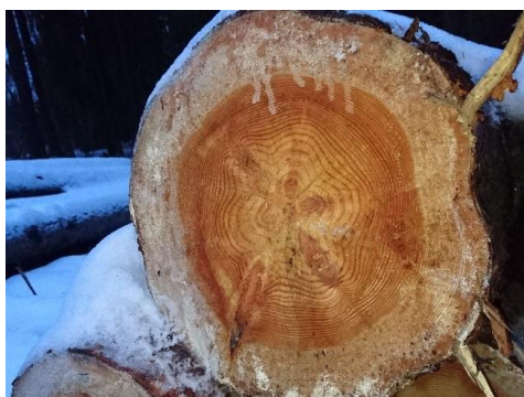
Figure 1. Heartwood and sapwood are visibly different in Scots pine.
